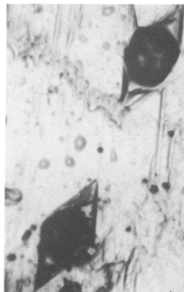
Figure 5 Two oriented, parallelogram-shaped growth hillocks with bulk impurity at the initiation centre, and tiny growth hillocks with distinct growth layers on a prism face of an AP crystal ( \times 200 ).
