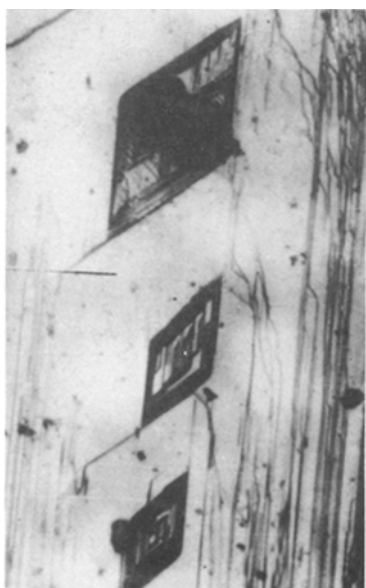
Figure 7 Well-defined isolated growth hillocks on a prism face of an AA crystal ( \times 200 ).
