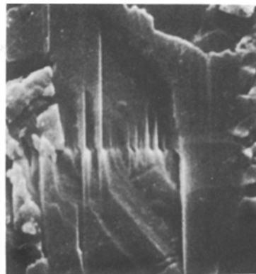
Figure 11 An eccentric etch pit on the prism face of an AA crystal ( \times 1200 ).
